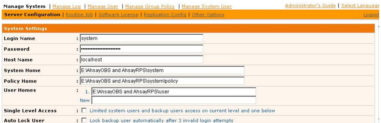
The screenshot shows the 'System Settings' page in the AhsayOBS web console. The 'Auto Lock User' checkbox is unchecked, indicating that the account lockout feature is disabled. The settings include:
